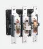
7. The contact system of the products with the rated current above 370 A adopts the structure that the arc contact and the conductive contact are separated. The arc contact adopts the multi-element copper-based contact with wear resistance and welding resistance, and the conductive contact adopts the silver-based contact with low resistivity and good conductivity, which greatly enhances the reliability of making and breaking.
